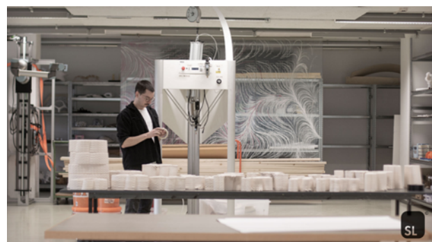
■ 3D tlačové experimenty s materiálom na báze hliny a mycelia na TU Grac zdroj: 3dwasp.com / 3D printing experiments with material based on clay and mycelium at TU Grac source: 3dwasp.com
